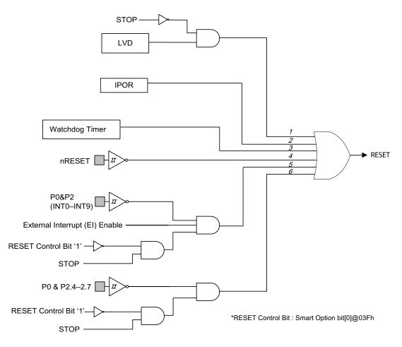
Figure 64. Reset Sources of the S3F80P9 MCU
