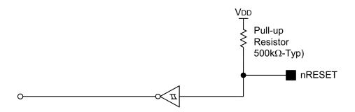
Figure 12. nRESET Pin Circuit, Type 7
