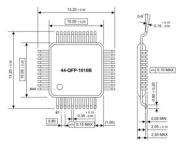
Figure 98. 44-pin QFP Package Dimensions
