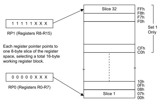
Figure 17. 8-Byte Working Register Areas
