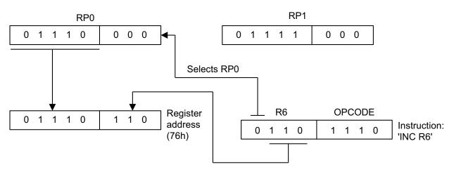
Figure 24. 4-Bit Working Register Addressing Example
