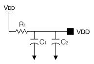
Figure 61. Power Circuit
