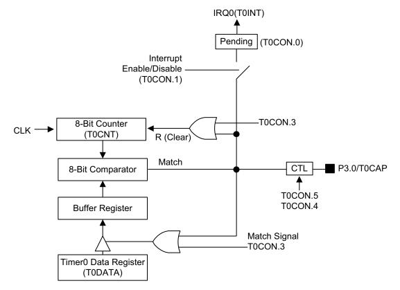
Figure 74. Simplified Timer 0 Function Diagram: Interval Timer Mode
