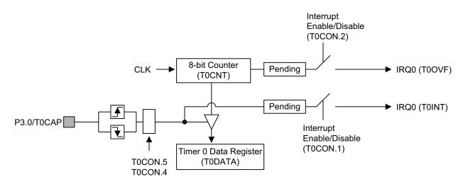
Figure 76. Simplified Timer 0 Function Diagram: Capture Mode
