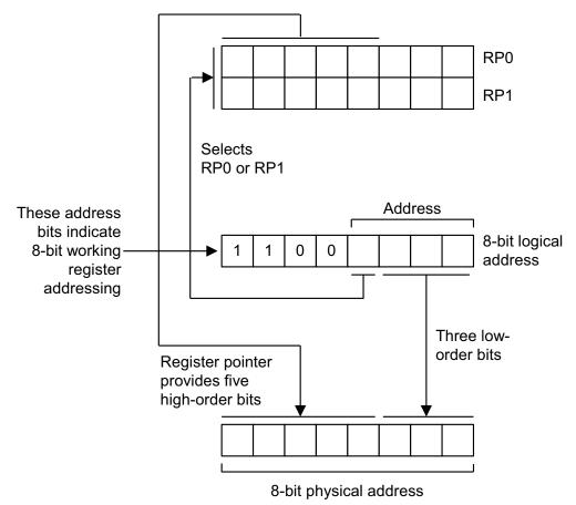
Figure 25. 8-Bit Working Register Addressing
