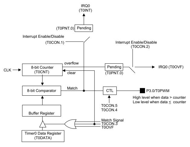
Figure 75. Simplified Timer 0 Function Diagram: PWM Mode
