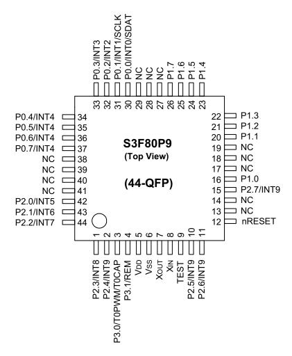
Figure 6. Pin Assignments, 44-Pin QFP Package
