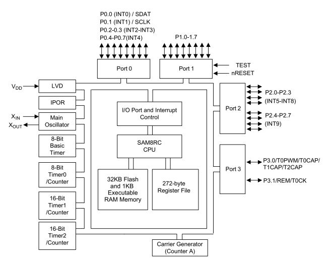
Figure 2. 44-pin QFP and 32-Pin SOP/QFN Block Diagram
