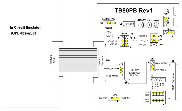
Figure 103. TB80PB Target Board Configuration
