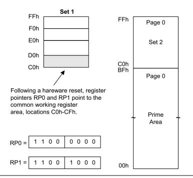
Figure 22. Common Working Register Area
