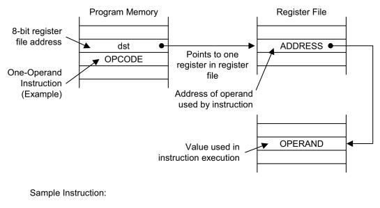
RL @SHIFT ; Where SHIFT is the label of an 8-bit register address.
