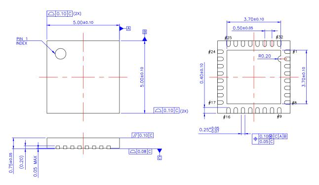
Figure 100. 32-Pin QFN Package Dimensions
