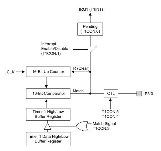
Figure 79. Simplified Timer 1 Function Diagram: Interval Timer Mode
