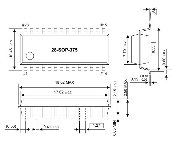
Figure 101. 28-Pin SOP Package Dimensions
