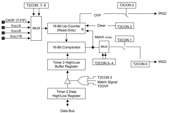
Figure 85. Timer 2 Block Diagram
