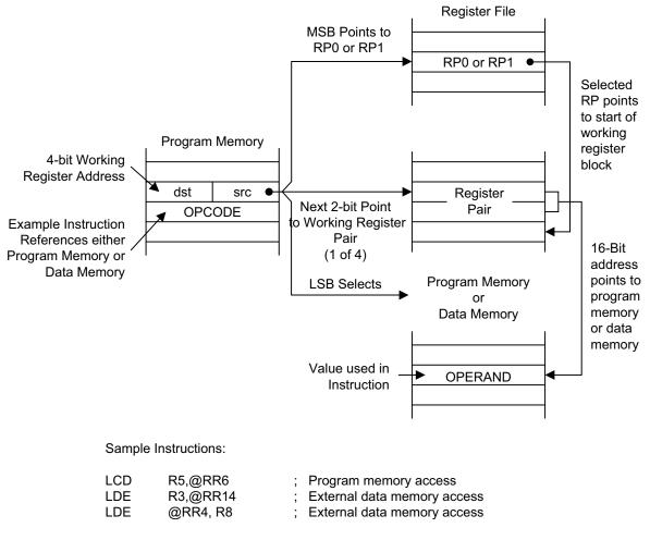
Figure 33. Indirect Working Register Addressing to Program or Data Memory
