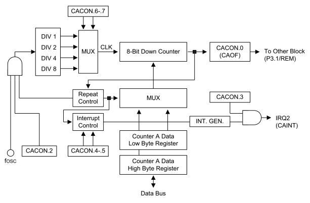
Figure 80. Counter A Block Diagram
