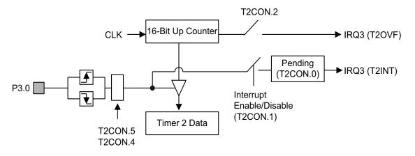
Figure 86. Simplified Timer 2 Function Diagram: Capture Mode
