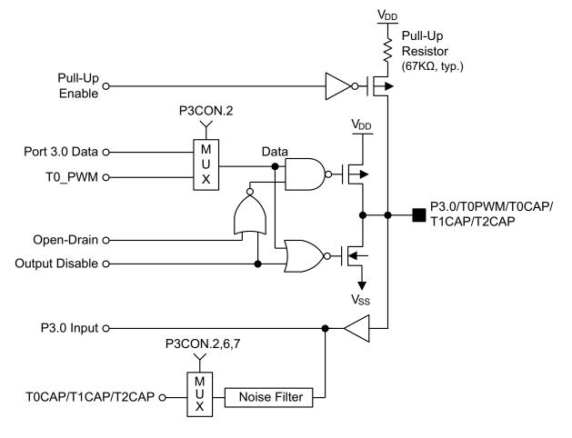
Figure 10. Port 3 Pin Circuit, Type 4
