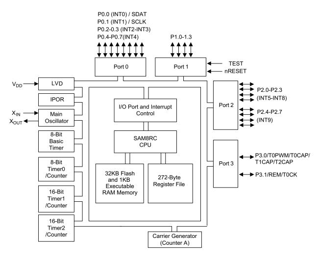
Figure 1. 28-Pin SOP Block Diagram
