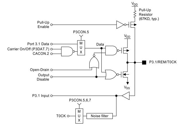
Figure 11. P3.1 Pin Circuit, Type 5
