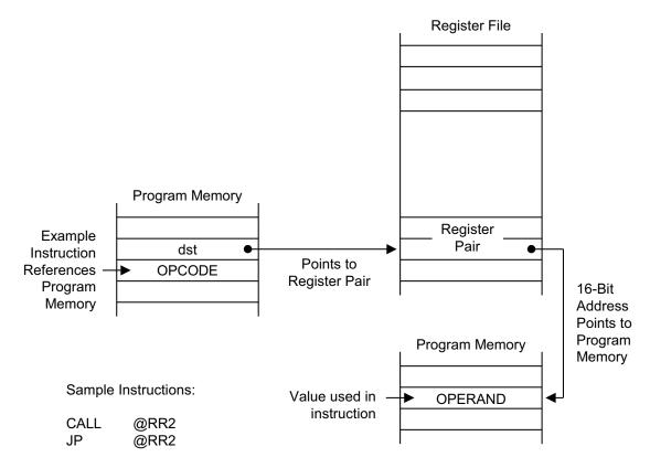
Figure 31. Indirect Register Addressing to Program Memory
