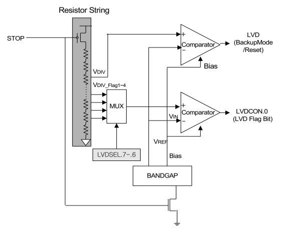
Figure 92. Low Voltage Detect Block Diagram
