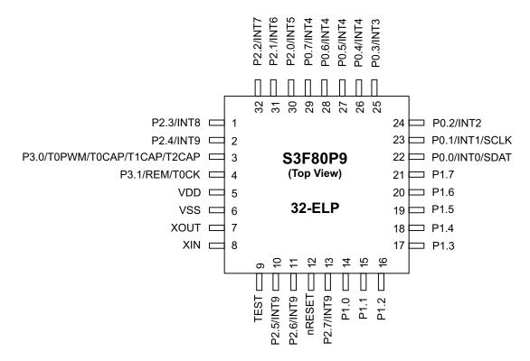
Figure 5. Pin Assignments, 32-Pin QFN Package
