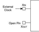
Figure 59. External Clock Circuit
