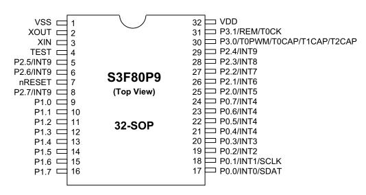
Figure 4. Pin Assignments, 32-Pin SOP Packages
