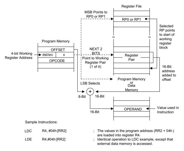
Figure 35. Indexed Addressing to Program or Data Memory with Short Offset
