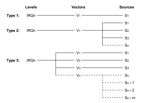
Figure 42. S3F8 Series Interrupt Types
