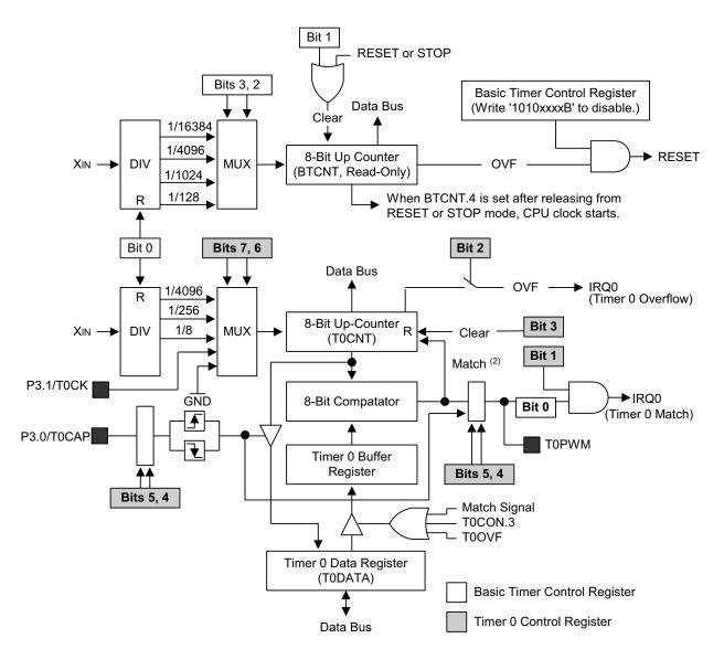
Figure 73. Basic Timer and Timer 0 Block Diagram
