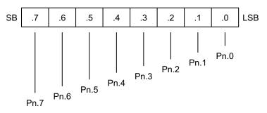
Figure 72. S3F80P9 I/O Port Data Register Format
