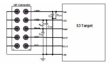
Figure 107. PCB Design Guide for In System Programming
