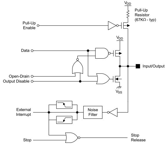
Figure 9. Port 2 Pin Circuit, Type 3
