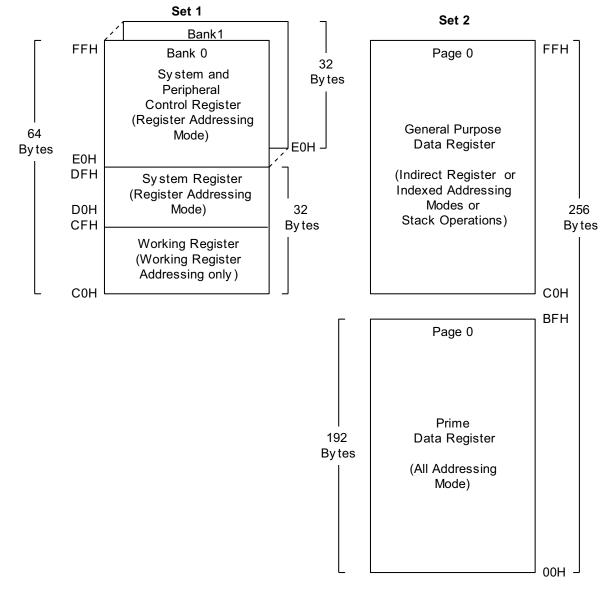
Figure 15 shows the organization of the Internal Register File.
