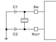
Figure 58. Main Oscillator Circuit
