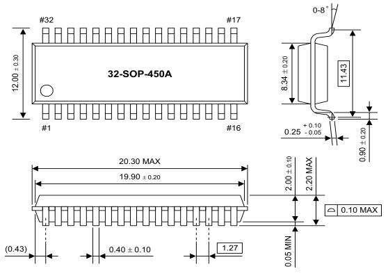
Figure 99. 32-Pin SOP Package Dimensions
