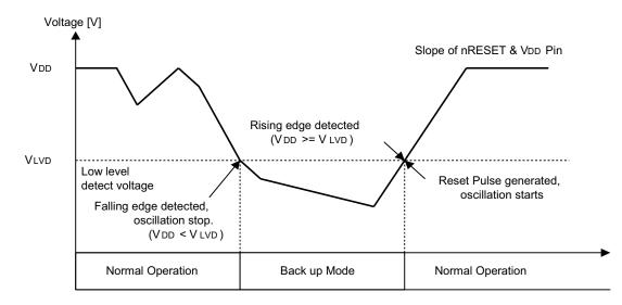
Figure 70. Timing Diagram for Backup Mode Input and Released by LVD
