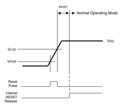
Figure 67. Timing Diagram for Internal Power-On Reset Circuit
