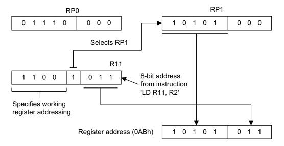
Figure 26. 8-Bit Working Register Addressing Example
