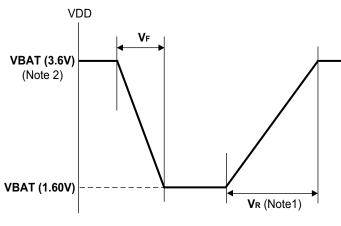
Figure 63. Chip Operating Voltage Guideline
