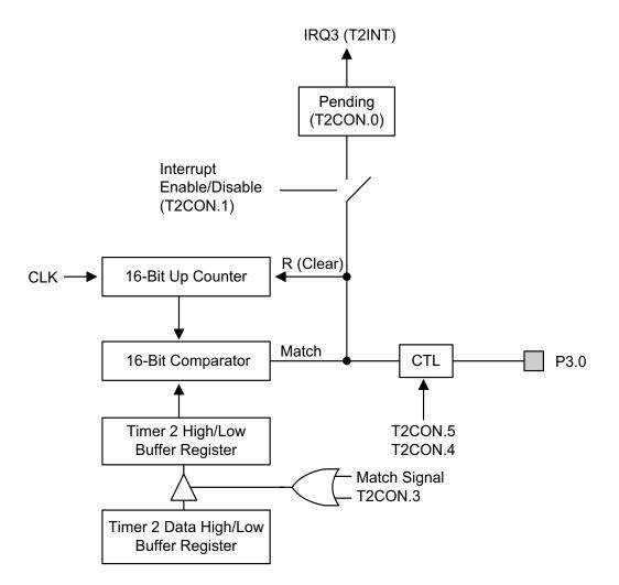
Figure 87. Simplified Timer 2 Function Diagram: Interval Timer Mode
