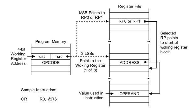
Figure 32. Indirect Working Register Addressing to Register File
